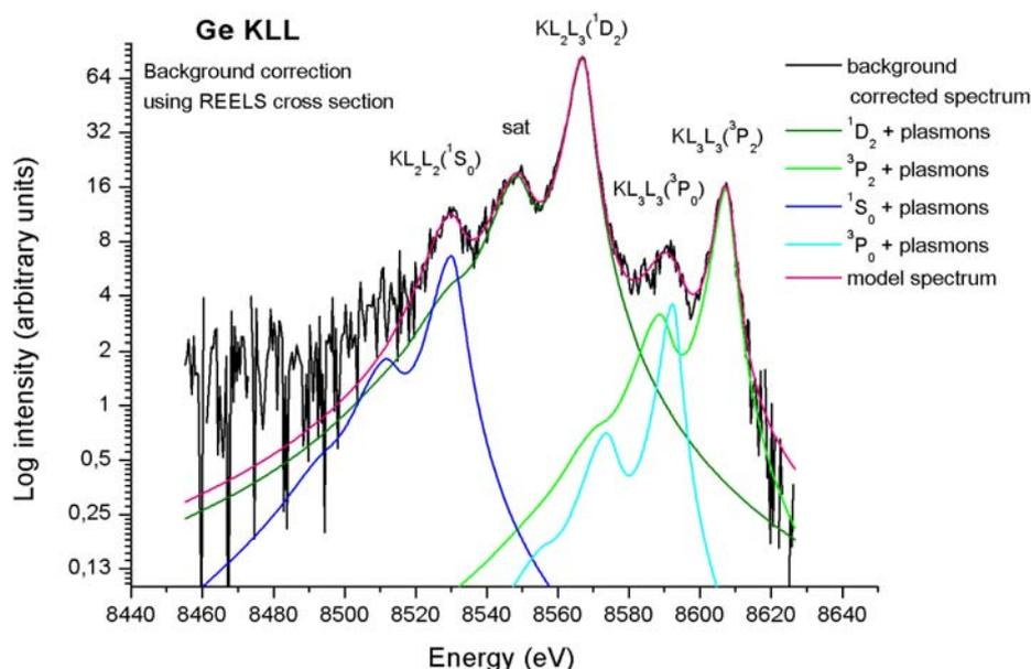
Fig. 1. The decomposition of the experimental Ge  $KL_{23}L_{23}$  spectrum photoexcited from a polycrystalline Ge layer of 100 nm thickness.
