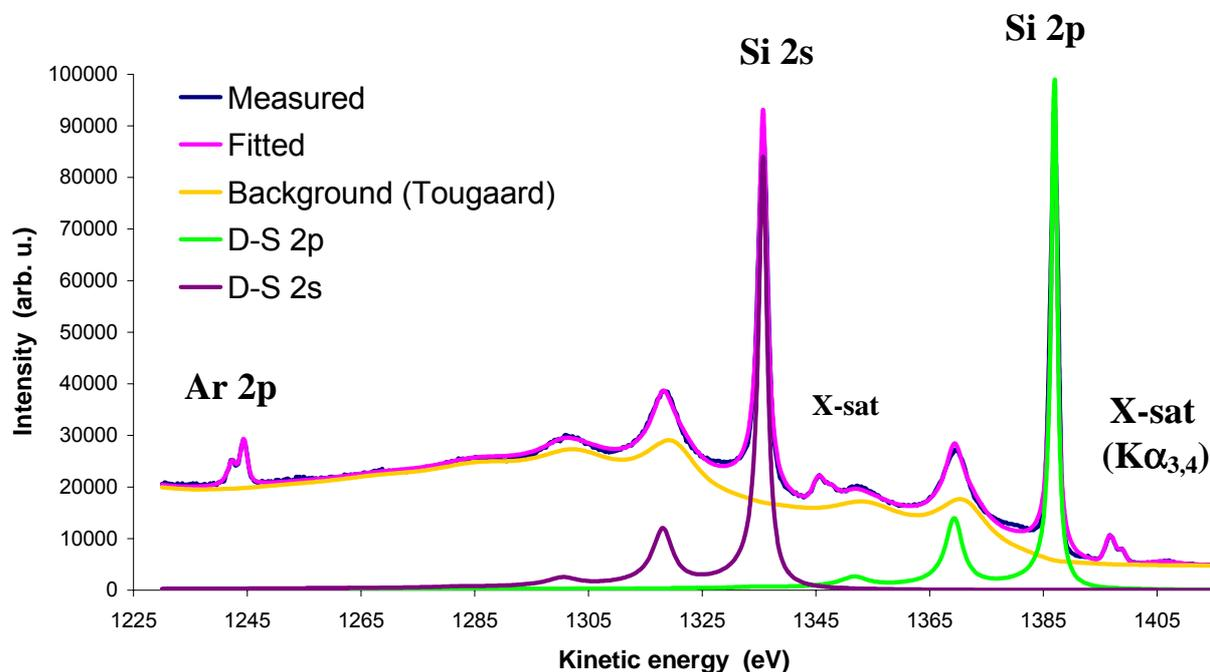
Fig. 3. The decomposition of the Si 2s, 2p photoelectron spectrum excited by Al K $\alpha$  X-rays from an amorphised single crystal sample.
