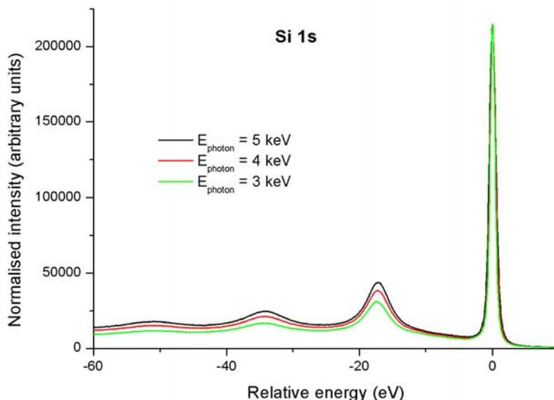
Fig. 2. Normalized Si 1s photoelectron spectra excited from a Si single crystal sample by monochromatized X-ray photons of 3, 4, and 5 keV, respectively.
